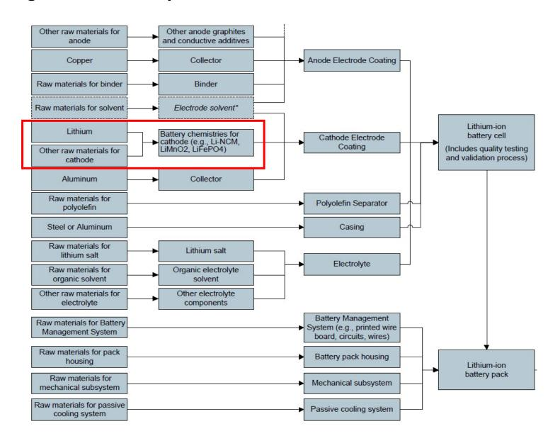
Cathode material is only a small part of the number of materials and components required for a Li-ion battery
