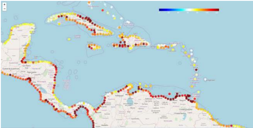
Map III.6 Central America, the Caribbean and northern South America: change of 0.5 m in vertical breakwater overtopping because of sea level rise, 2040 (Percentages)
